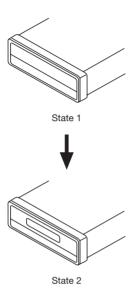
2. Press ७ (power) button to turn on the unit. Then press △ (eject) button, the panel will turn down to horizontal position (see State 3).
